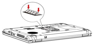
Figure 8-7 Pushing the memory module down
